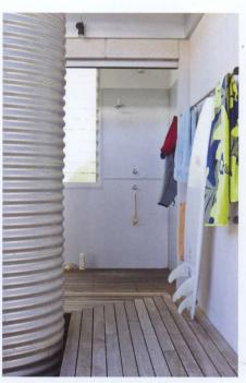
The owners bucked trends and opted for a one bathroom house. The water from the shower runs through the timber slats and into a waterproof tray, which then drains to the worm farm waste system. Twelve metres of copper piping was installed for hanging towels, instead of 12 separate towel racks. Copper piping is easily recycled, and is in high demand at recycling centres.
